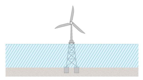
Figure 3.5: Illustrative jacket (suction bucket) foundation design.
