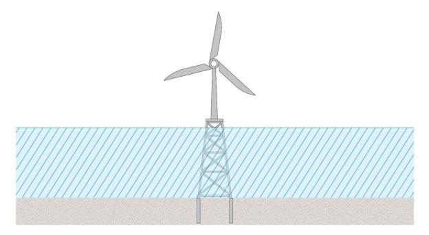
Figure 3.4: Illustrative jacket (pin pile) foundation design.
