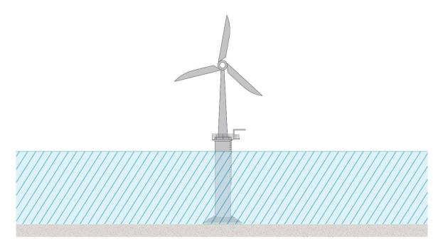
Figure 3.3: Illustrative monopile foundation design.
