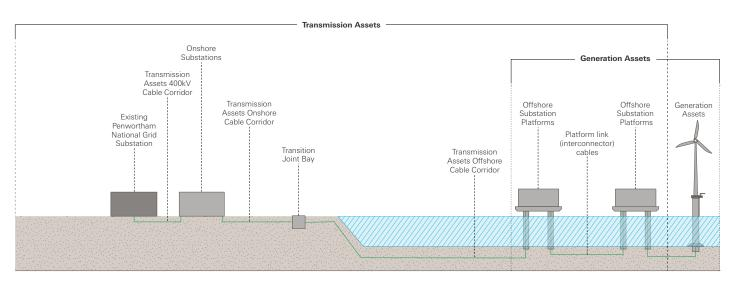
This indicative diagram illustrates which part of the projects are classified as Generation Assets (Morecambe Offshore Windfarm and Morgan Offshore Wind Project) and which parts are classified as Transmission Assets (Morgan and Morecambe Offshore Wind Farms: Transmission Assets).
